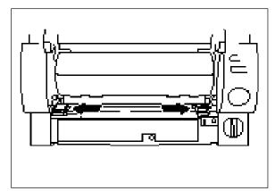
(6) Slide the new side cutter to secure it in the side cutter holder.
